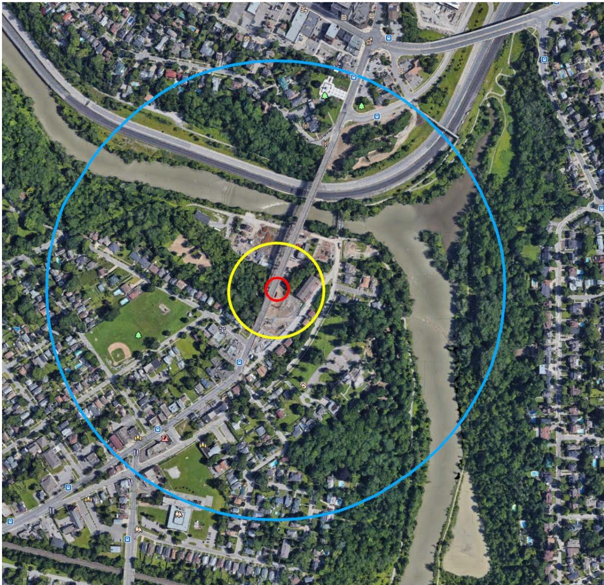
Figure 6: Approximate zones of influence based on 25 mm/s (red), 5 mm/s (yellow), and 0.5 mm/s (blue) PPV thresholds for a hypothetical pile driving operation (centre of concentric circles).
