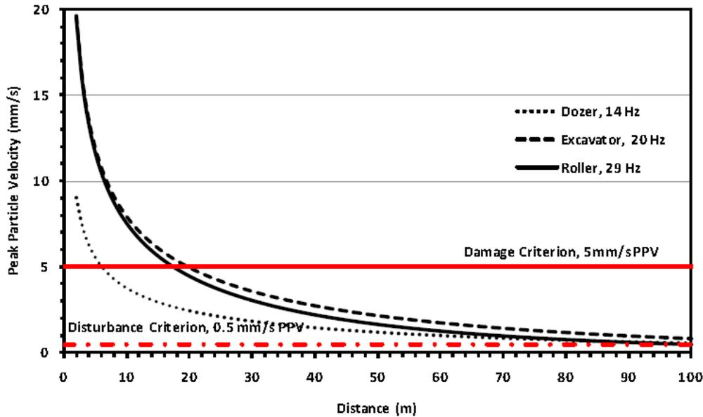
Figure 5: Expected peak particle velocities for Class III soils (Source: Cenek et al 2012)
