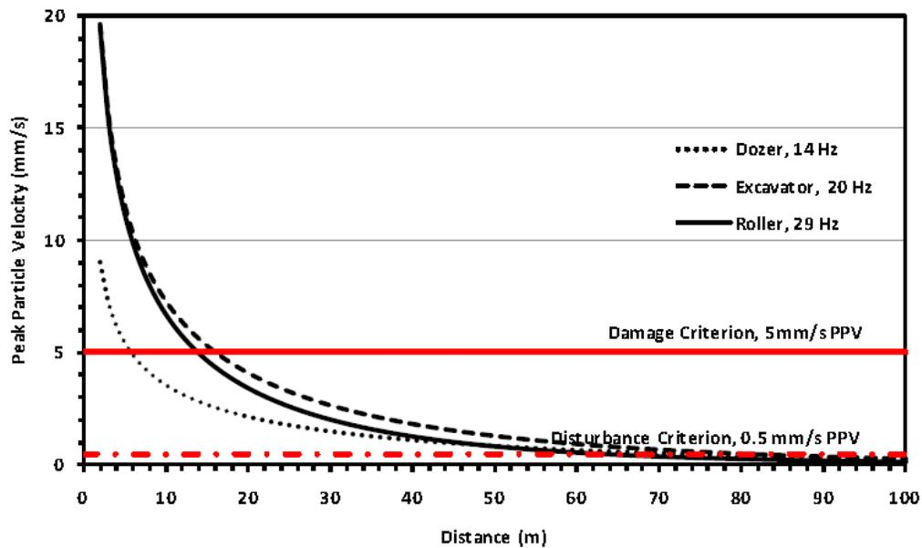
Figure 4: Expected peak particle velocities for Class II soils (Source: Cenek et al 2012)
