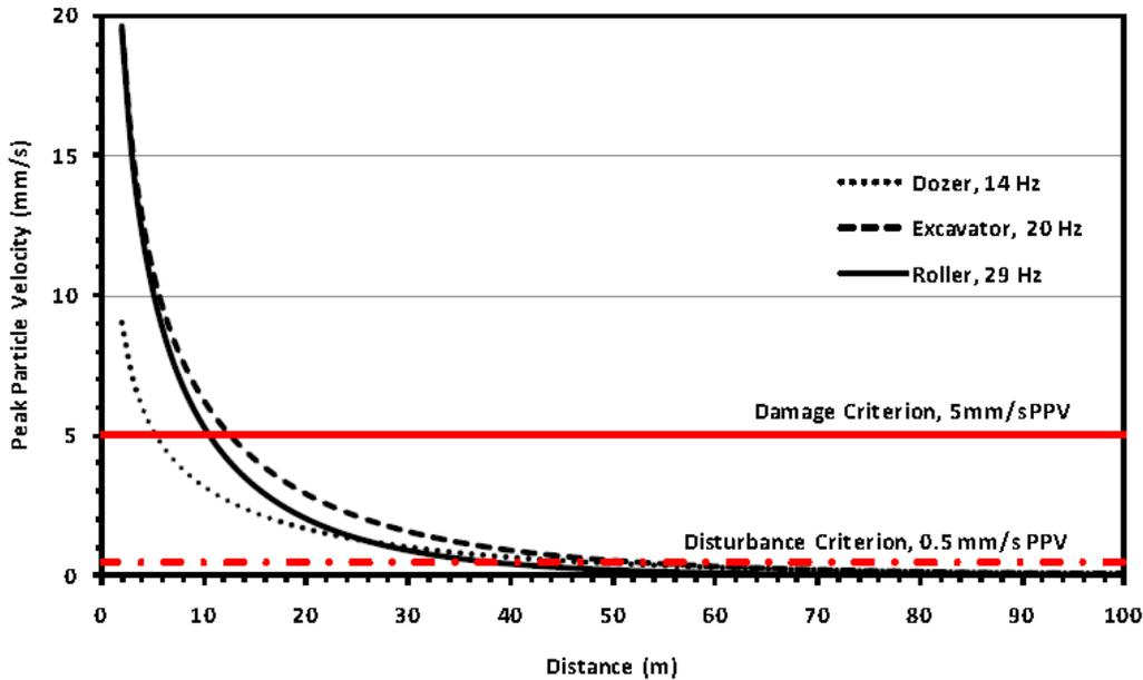
Figure 3: Expected peak particle velocities for Class I soils (Source: Cenek et al 2012)
