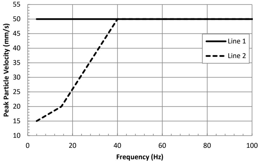
Figure 1: Transient vibration limits in BS 7358-2:1993
