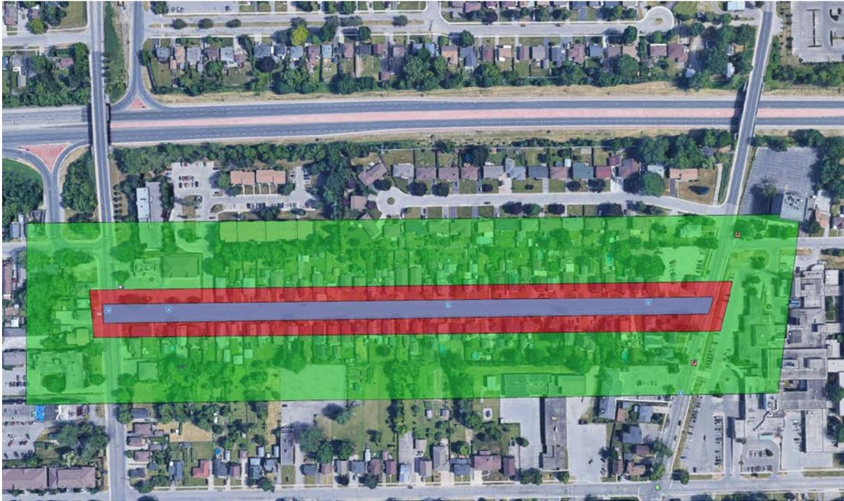
Figure 7: Approximate zones of influence based on 5 mm/s (red) and 0.5 mm/s (green) vibration thresholds for a hypothetical road replacement project (middle blue).
